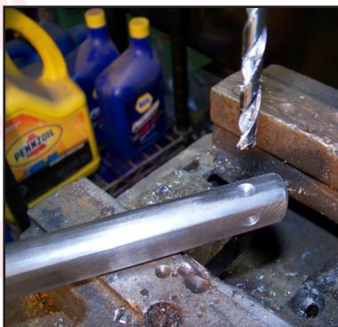
use a  $\frac{1}{4}$  inch drill bit and create a relief for the setscrew. This relief only needs to be approximately  $\frac{3}{16}$  inch deep.
