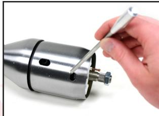
Make sure your road wheels are pointing straight forward and your column and all mounts are completely secure. Next install your OEM wheel with all of the original components or add an aftermarket wheel with an adaptor. Slide the wheel on top of the splined top shaft of the column. You may need to adjust your wheel a little to fit into the splines. Place wheel nut on top of wheel and torque wheel nut to 35lbs.
