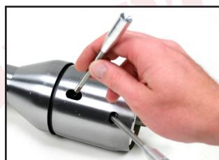
The turn signal lever (longer of the two levers) is installed into the threaded hole closest to the top of the column.
