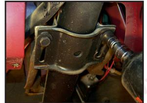
4.) Tighten the dash and firewall mounts to the vehicle securely.
