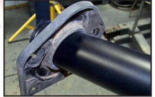
2.) **A. 2 wheel drive:** From inside the truck slip the column into the rag joint. Then loosely install the bolts through the dash mount and into the dash. It may be necessary to move the column in or out slightly to install the pinch bolt on the rag joint. Tighten the rag joint bolt before tightening the column dash bolts. Make sure the rag joint is not put under stress, the rubber part of the rag joint should be flat and not pushed or pulled by the column.
