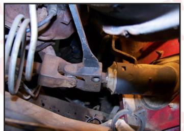
7.) Once the column has been removed from your vehicle, remove the firewall mount and original seal. Place them off to the side as you will be reusing these when installing the new column. You may want to clean these items and repaint them prior to re-installation. Since this seal is stopping fumes and water from coming in the cab inspect it and replace it if they are cracked or damaged in anyway.
