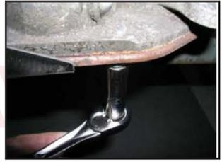
14. Make sure the transmission is in Park. Install the transmission shift lever using the supplied nut and bolt. Next, install the kick down lever with the original nut and washer as shown.
