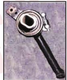
6. Reinstall the horseshoe bracket. It can either go on the top side of the column or below, it is your choice. Check for any brake pedal interference.
