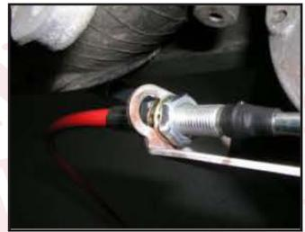
15. Try to shift the column. You may experience a tight pattern, if so; slightly loosen the bracket around the column. This should allow the column to move easier. If not, check that the cable is in alignment from the bracket to the lever.
