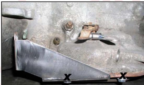
12. On the 727/904 Chrysler transmission you must remove the original shift lever and kick down lever. Remove the two pan bolts marked with X's in the picture above and install the bracket towards the front of the transmission.
