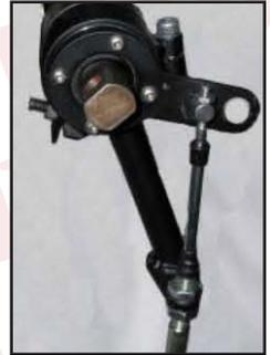
26. Try to shift the column. You may experience a tight pattern, if so; slightly loosen the bracket around the column. This should allow the column to move easier. If not, check that the cable is in alignment from the bracket to the lever. Remember to check the transmission fluid levels and add more fluid if necessary.
