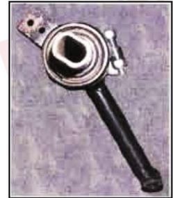
22. Reinstall the horseshoe bracket. It can either go on the top side of the column or below, it is your choice. Check for any brake pedal interference.
