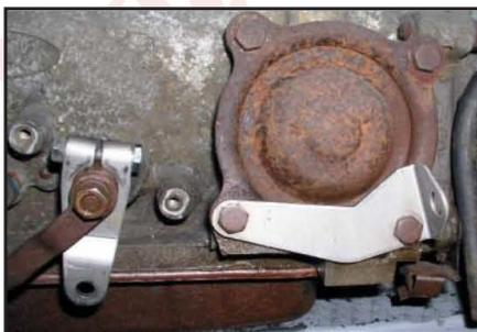
13. Take the small nut, two rubber boots, and one large nut and washer off the transmission end of the cable. Insert the cable into the bracket. Reinstall the large washer and nut and two boots. Rotate the shift lever clockwise to the Park position. Now you are going to put the swivel onto the threaded end of the cable and turn it until it lines up with the hole of the shift lever.
