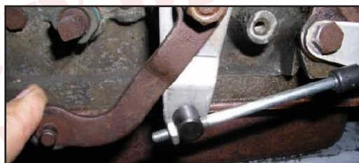
14. Try to shift the column. You may experience a tight pattern, if so; slightly loosen the bracket around the column. This should allow the column to move easier. If not, check that the cable is in alignment from the bracket to the lever.
