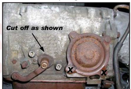
the nut and washer from the kick down lever and then remove the kick down lever itself.
