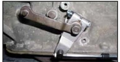
15. Try to shift the column. You may experience a tight pattern, if so; slightly loosen the bracket around the column. This should allow the column to move easier. If not, check that the cable is in alignment from the bracket to the lever.
