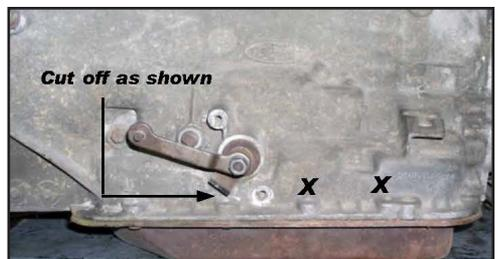
x's. Also remove the nut and washer from the kick down lever and then remove the kick down lever itself.
