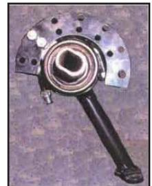
will need to take the small nut and rubber boots off. Insert the cable through the bottom side of the bracket and reinstall the large nut, washer and boots. Try to center the nuts and washers on the available threads. *You will see why this is important in a later step.*
