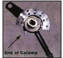
5. Put the column into the park position. Install the two piece bracket on the column toward the firewall side of the lower shift lever. Make sure that the hole that the cable will pass through faces forward. Make it snug but do not tighten completely as you may have to move it later.
