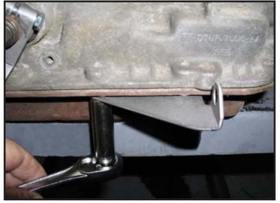
13. Make sure that the transmission is in Park. Install the transmission shift lever using the supplied nut and bolt. Note that it covers the original shift lever previously cut off. Next, install the kick down lever with the original nut and washer as shown. Install the cable bracket and the two bolts as shown.
