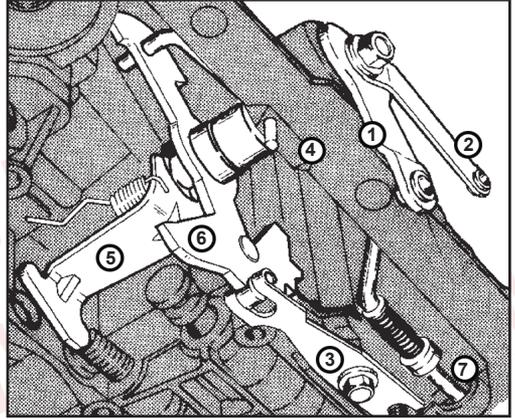
1. Remove the pan and disconnect the old shift linkage from the transmission shift lever. (1)
