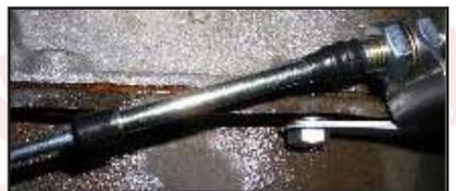
rubber boots back onto the end of the cable.
