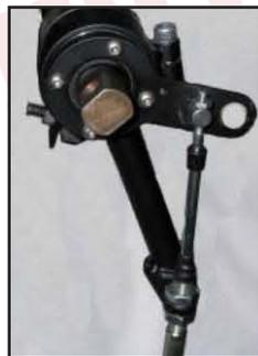
17. Reinstall the shift lever as close to the swivel as possible. Now, you could turn the bracket or loosen the large nut and adjust so the swivel goes into the 5/16" hole that you drilled in the shift arm. Insert the cotter pin in swivel, tighten large nut and bolt on bracket. Do not tighten so much that it squeezes the delrin bushing in the bottom of the column. Doing so could make it hard to shift. Remember, the cable has to be pushed down completely.
