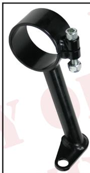
12. Loosen the nut and bolt on the cable bracket so that the clamp loosens a little. Slide the clamp on the column with the small end at appx. 5 o'clock (looking down from the top of the column.) The hole on the small end of the clamp should face the front of the vehicle. **DO NOT** tighten yet!
