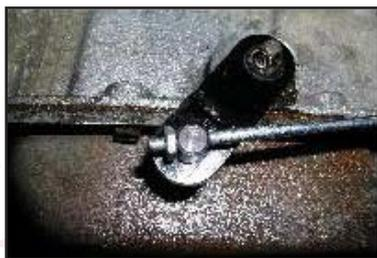
**Note:** Swivel may have to be adjusted one turn in either direction. Install the cotter pin supplied with the kit into the swivel and spread the pins ends. Move the transmission selector back into the Park position.
