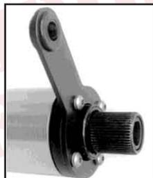
13. The gearshift lever will need a hole drilled exactly  $1\frac{29}{32}$ " or 1.906" from the center of the large hole towards the linkage hole, in the center of the shift lever arm. The hole should be  $\frac{5}{16}$ " or .312 in diameter, no larger.
