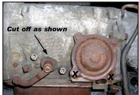
10. Make sure that the transmission is in Park. Install the transmission shift lever using the supplied nut and bolt. Next, install the kick down lever with the original nut and washer as shown. Install the cable bracket and the two bolts as shown.
