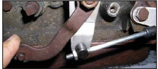
12. Try to shift the column. You may experience a tight pattern, if so; slightly loosen the bracket around the column. This should allow the column to move easier. If not, check that the cable is in alignment from the bracket to the lever.
