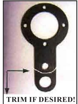
5. The next step will be to install the cable. You will notice that both ends are the same. In order to get one large nut and washer off the shift cable, you will need to take the small nut and rubber boots off. Insert the cable through the bottom side of the bracket and reinstall the large nut, washer and boots. Try to center the nuts and washers on the available threads. You will see why this is important in a later step.
