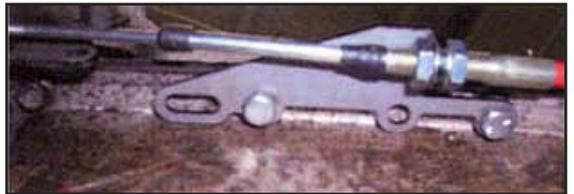
10. The two transmission pan bolts could be either Metric or American threads. You will need to purchase two bolts 1/4" longer than the two that you removed. Spacers need to be placed between the bracket and the transmission pan with the two longer bolts holding it all together in the holes of the bracket as shown.
