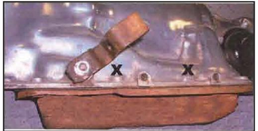
9. Looking at the side of the transmission, remove the stock shift lever and the two pan bolts marked with X's.
