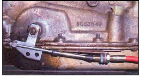
travel, loosen the large nuts and washers and move the cable forward or backward to gain more travel. Then retighten the large nuts and washers. Install the small nut and tighten.
