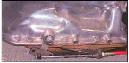
13. Try to shift the column. You may experience a tight pattern, if so slightly loose the bracket around the column. This should allow the column to move easier. If not check that the cable is in alignment from the bracket to the lever.
