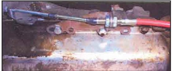
10. The two transmission pan bolts could be either Metric or American threads. You will need to purchase two bolts 1/4" longer than the two that you removed. Spacers need to be placed between the bracket and the transmission pan with the two longer bolts holding it all together in the holes of the bracket as shown.
