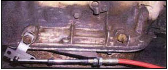
pin. If it needs more travel, loosen the large nuts and washers and move the cable forward or backward to gain more travel. Then retighten the large nuts and washers. Install the small nut and tighten.
