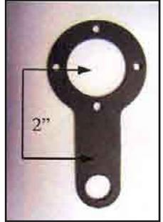
3. The gearshift lever will need a hole drilled exactly 2" from the center of the large hole towards the linkage hole, in the center of the shift lever arm. The hole should be 5/16" or .312 in diameter, no larger!
