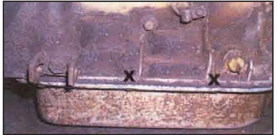
9. Looking at the side of the transmission, remove the stock shift lever and the two pan bolts marked with X's. Save the nut and washer from the shift lever and the two pan bolts.
