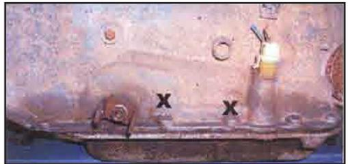
9. Looking at the side of the transmission, remove the stock shift lever and the two pan bolts marked with X's. Save the nut and washer from the shift lever and the two pan bolts.
