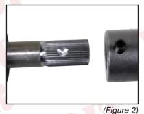
While holding the column have your helper install the setscrews into the coupler. Next gently tighten them onto the column & then loosen and remove the setscrews. Doing this will mark the spot where you need to drill the shaft! Now remove the column out of the vehicle and spot drill a dimple into the shaft with the same 5/16 drill bit approximately 1/8 of an inch deep. This should be just past the bottom of the spline depth.
