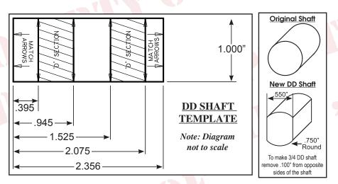
Starting from an 1/8 from the bottom, wrap the paper template around the shaft and match the horizontal arrows together.
