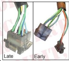
The early group had two connectors, one with 6 wires and one with 2 wires. The later had the same 8 wires, but all in one connector.
