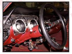
Remove the nut and use a wheel puller to pull the original steering wheel off the original column. (Figure 2)
