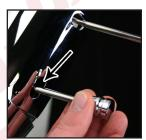
and adaptor removed, look down from the top of the column and you'll see two holes on the turn signal switch. One is D shaped and the other is round. With the lever in place, insert the provided screw into the **round** hole. Use a #2 Phillips screw driver to tighten the screw tightly.
