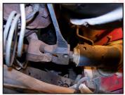
7.) Once the column has been removed from your vehicle, remove the firewall mount and original seal. Place them off to the side as you will be reusing these when installing the new column. You may want to clean these items and repaint them prior to re-installation. Since this seal is stopping fumes and water from coming in the cab inspect it and replace it if they are cracked or damaged in anyway.
