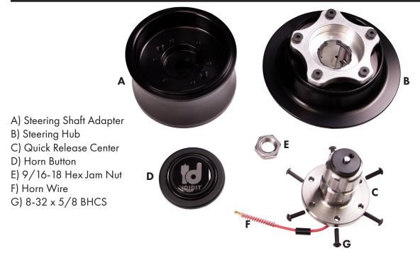
IDIDIT'S line of quick release steering hubs are designed for GM OE or IDIDIT GM style shaft. Installation should be done by a trained professional.
