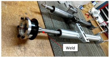
Figure 1: quick release steering hub shown on Ididit racing column.
