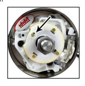
the horn button. If there is not a hole in adaptor to ground to, use one of the puller holes with a short bolt to attach the wire to the adaptor.
