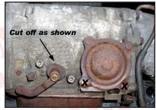
the nut and washer from the kick down lever and then remove the kick down lever itself.
