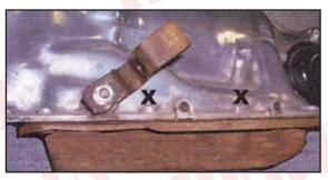
12. The two transmission pan bolts could be either Metric thread or American thread. You will need to purchase two bolts 1/4" longer than the two that you removed. Spacers need to be placed between the bracket
