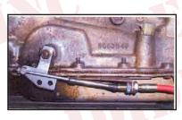
you are going to put the swivel onto the threaded end of the cable and turn it until it lines up with the forward hole of the shift lever. Install the cotter pin. If it needs more travel, loosen the large nuts and washers and move the cable forward or backward to gain more travel. Then retighten the large nuts and washers. Install the small nut and tighten.
