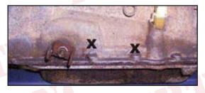
12. The two transmission pan bolts could be either Metric thread or American thread. You will need to purchase two bolts 1/4" longer than the two that you removed. Spacers need to be placed between the bracket and the transmission pan with the two longer bolts holding
