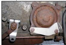
11. Take the small nut, two rubber boots and one large nut and washer off the transmission end of the cable. Insert the cable into the bracket. Reinstall the large washer and nut and two boots. Rotate the shift lever clockwise to the Park position. Now you are going to put the swivel onto the threaded end of the cable and turn it until it lines up with the hole of the shift lever. Install the cotter
