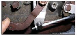
pin. If it needs more travel loosen the large nuts and washer and move the cable forward or backward to gain more travel. Then retighten the large nuts and washers. Install the small nut and tighten.
