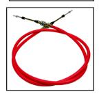
6. Push the cable down through its outer cover so that it will be as short as possible. Put the column in Park. Now, figure out where you want the bracket to be, 5 o'clock will probably be a good place. Install the swivel on the small thread and turn it until it is centered on the thread. Now, install the small nut and turn it until it bottoms out on the swivel. DO NOT tighten yet!
