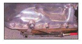
cotter pin. If it needs more travel, loosen the large nuts and washers and move the cable forward or backward to gain more
