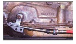
travel, loosen the large nuts and washers and move the cable forward or
