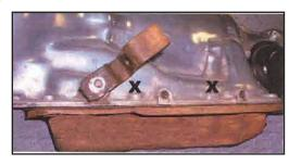
Looking at the side of the transmission, remove the stock shift lever and the two pan bolts marked with X's.
