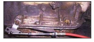
pin. If it needs more travel, loosen the large nuts and washers and move the cable forward or backward to gain more travel. Then retighten the large nuts and washers. Install the small nut and tighten.
