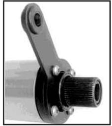
2. Loosen the nut and bolt on the cable bracket so that the clamp loosens a little. Slide the clamp on the column with the small end at appx. 5 o'clock (looking down from the top of the column.) The hole on the small end of the clamp should face the front of the vehicle. DO NOT tighten yet!
