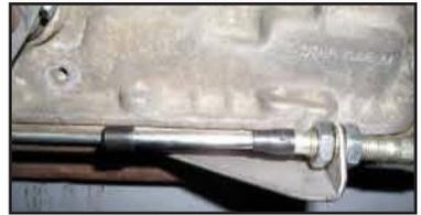
13. Try to shift the column. You may experience a tight pattern, if so; slightly loosen the bracket around the column. This should allow the column to move easier. If not, check that the cable is in alignment from the bracket to the lever.
