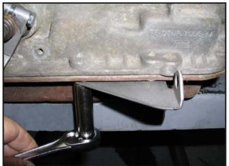
11. Make sure that the transmission is in Park. Install the transmission shift lever using the supplied nut and bolt. Next, install the kick down lever with the original nut and
