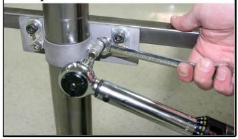
This dash mount is specifically designed for the ididit collapsible series of steering columns. It is critical to the system that these mounts have all fasteners torqued to the correct specifications. It is equally important that this item is not soaked in any corrosive materials i.e. rust removers or solvents.
