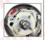
be sure). This is normally used when an o-ring is used to hold the button in place. The o-ring does not provide sufficient ground, therefore, an additional wire is provided to ground the horn button. If there is not a hole in adaptor to ground to, use one of the puller holes with a short bolt to attach the wire to the adaptor.
