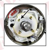
is provided to ground the horn button. If there is not a hole in adaptor to ground to, use one of the puller holes with a short bolt to attach the wire to the adaptor.
