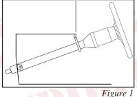
Attaching your column to a steering gearbox or rack & pinion system may require some combination of u-joints, couplers and shafts.
