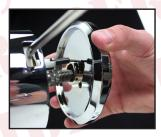
and slide it onto the column. A nut has been provided with your steering column. The nut will secure the wheel to the top of the column. The nut on the wheel should be torqued to 35 ft lbs.
