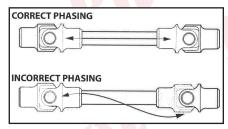
Sometimes if the u-joints are at a severe angle, even if they are phased correctly, a hard spot in the steering may occur for no apparent reason. If this happens, index the u-joints two or three splines in one direction. The hard spot should disappear or be minimized.
