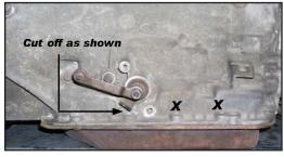
bolts marked with X's. Also remove the nut and washer from the kick down lever and then remove the kick down lever itself.
