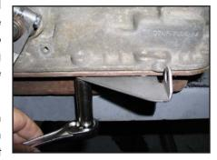
and bolt. Next, install the kick down lever with the original nut and
